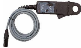
Current clamp 30/300 A power supplied from the instrument with extension 5 m (16.4 ft)
